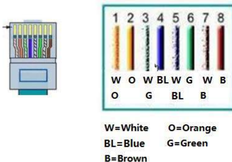
Appendix Figure 8-1 RJ-45 definition
