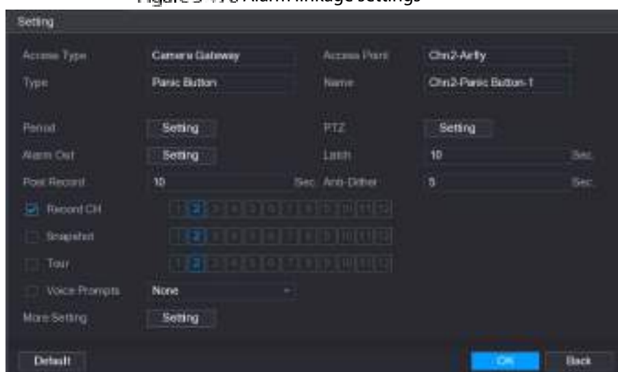
Figure 5-176 Alarm linkage settings
